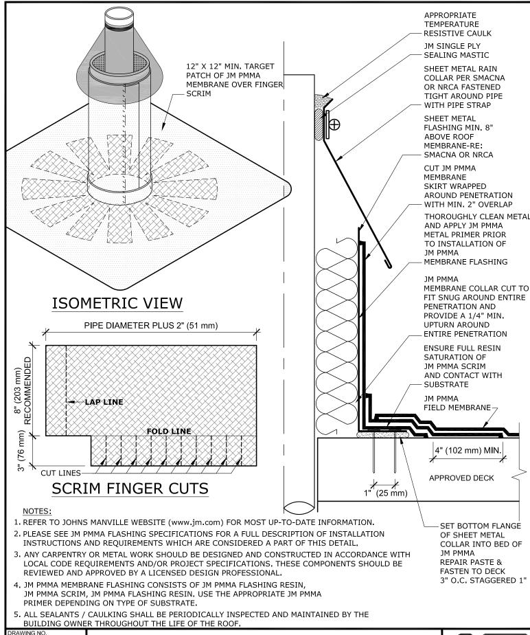
\_-FP-02 MEMBRANE TYPE: DRAINS & VENTS JM PMMA
