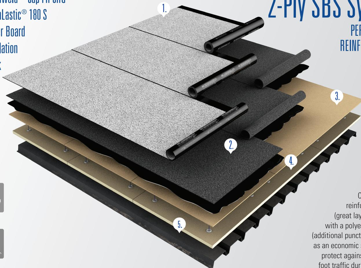
Combine a glass reinforced cap sheet (great lay-flat attributes) with a polyester base sheet (additional puncture resistance) as an economic solution to help protect against damage from foot traffic during installation.
