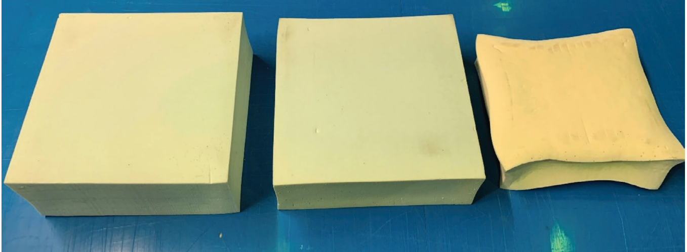
Figure 8: Post ASTM D2126 test samples of spray foam from left to right. JM Corbond III 7-inches (sprayed in four, immediate 1.75-inch passes), JM Corbond III 5-inches (sprayed in a single pass), and Product A high lift (5 inches in a single pass).
