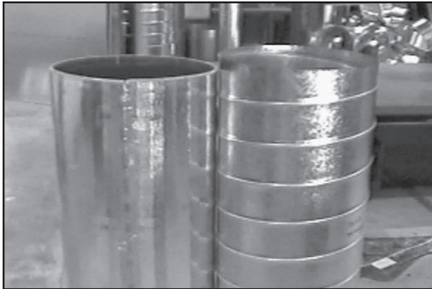
Figure 5-6. Formed liner and spiral duct
