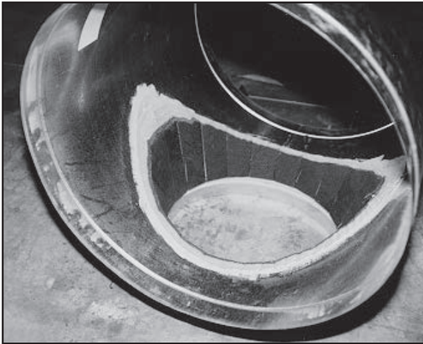
Figure 9-10. Finished contour cut
