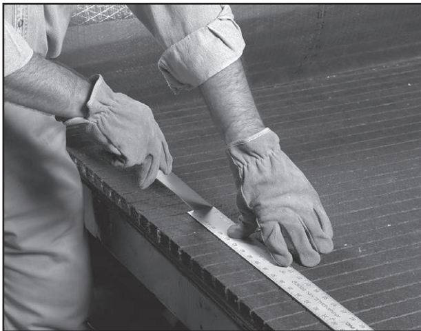
Figure 5-14. Measuring for stretchout
