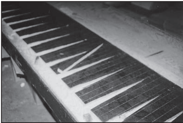
Figure 9-3. Liner board on bench with V-notches
