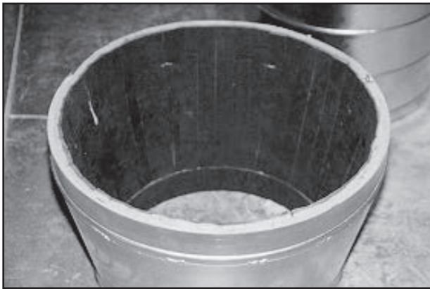
Figure 8-7. Taper insert in duct
