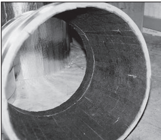
Figure 8-8. Finished taper section
