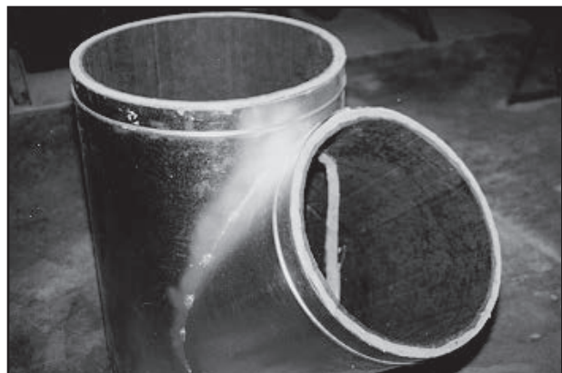
Figure 9-1. Angled tap on straight-through body
