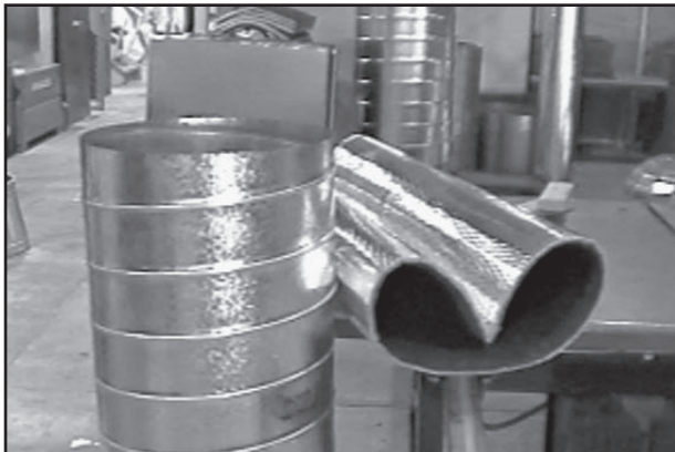
Figure 5-7. Liner folded inward
