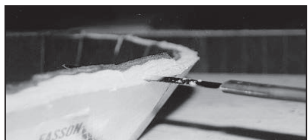
Figure 8-16. Trimming the insert
