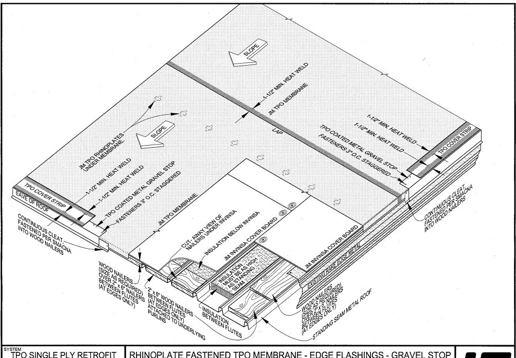
TPO SINGLE PLY RETROFIT **OVER STANDING SEAM METAL ROOF** (RHINOPLATE)
