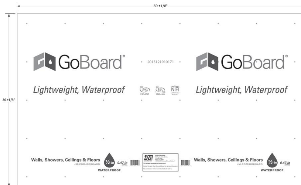
FIGURE 6—GOBOARD® 36-INCH X 60-INCH SHEET DIMENSIONS (1/2-INCH GOBOARD® IS SHOWN AS AN EXAMPLE; DIMENSIONS ARE THE SAME FOR 1/4-INCH AND 1/2-INCH)
