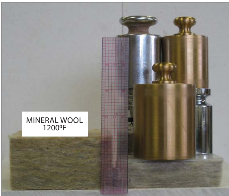
Figure 4 - The mineral wool on the left side of the photo is unconditioned.
