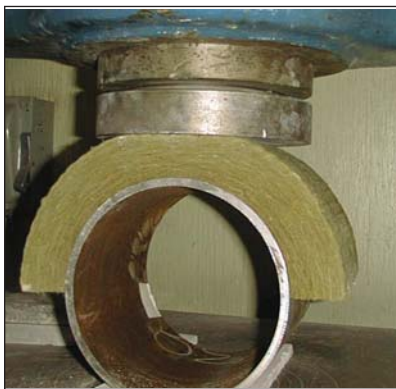
Figure 3 - Change in insulation thickness when a 120 pound load is applied.
