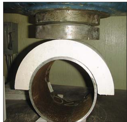
Figure 3 - Change in insulation thickness when a 120 pound load is applied.
