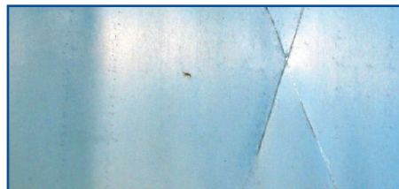
3000 series aluminum with POLYFILM - no corrosion
