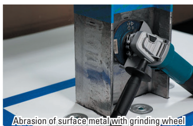
Abrasion of surface metal with grinding wheel
