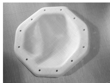
Prototype rear differential cover thermoformed from Neomera™ NCF-6 Series organosheet. Courtesy of University of Maine
