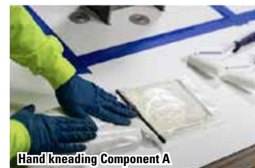
Hand kneading Component A
